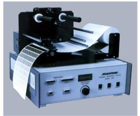
The ATLANTEK Model 200 thermal response test system is designed to provide thermal response vs. print density for imaging on direct thermal or thermal transfer media. This system is based on a special purpose ATLANTEK controller board which drives a standard thermal printhead and a programmable stepping drive controller.
